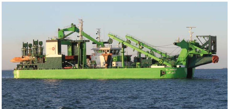
"Al Jarraf" will be able to discharge dredged material through a floating pipeline and directly into a barge
